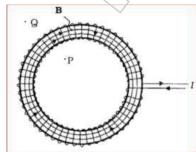
Toroid is a hollow circular ring on which a large number of turns of a wire are closely wound.
