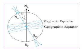
A vertical plane passing through the magnetic axis of a freely suspended magnet is called the magnetic meridian.
