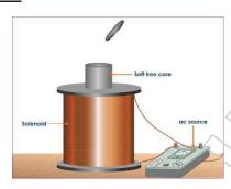
When a metallic disc is placed on one end of a solenoid connected to an ac source and with a soft iron core in it, the disc is thrown up into air.
