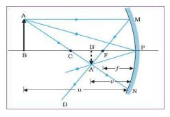
• In the diagram the two right-angled triangles A'B'F and MPF are similar.
