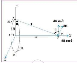
• The magnetic field at P due to the current element dl, at A is
